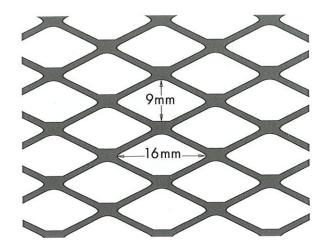
Expanded Reinforcement Coil has numerous applications in all types of building where additional strength is required within the coarse work. Used regularly to reduce cracking within brick and block masonry, coil mesh when embedded in the mortar joint, forms an integral structure of great tensile strength which will assist in the resistance to stresses, vibrations and thermal changes.
