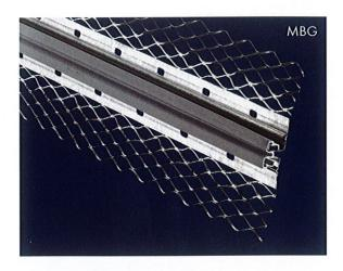
Cornercare Movement Bead provides a solution to thermal movement in plaster and rendered finishes. When placed vertically at predetermined centres provides a 6mm movement reducing the possibility of cracking. The face of the extrusion is covered by a Black PVC tape; to be removed when the plaster or render work has been completed.
